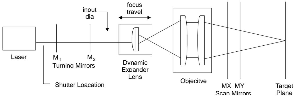
The beam shutter should be installed between the laser head and the Scan Head. The following figure shows the recommended location of the shutter.
