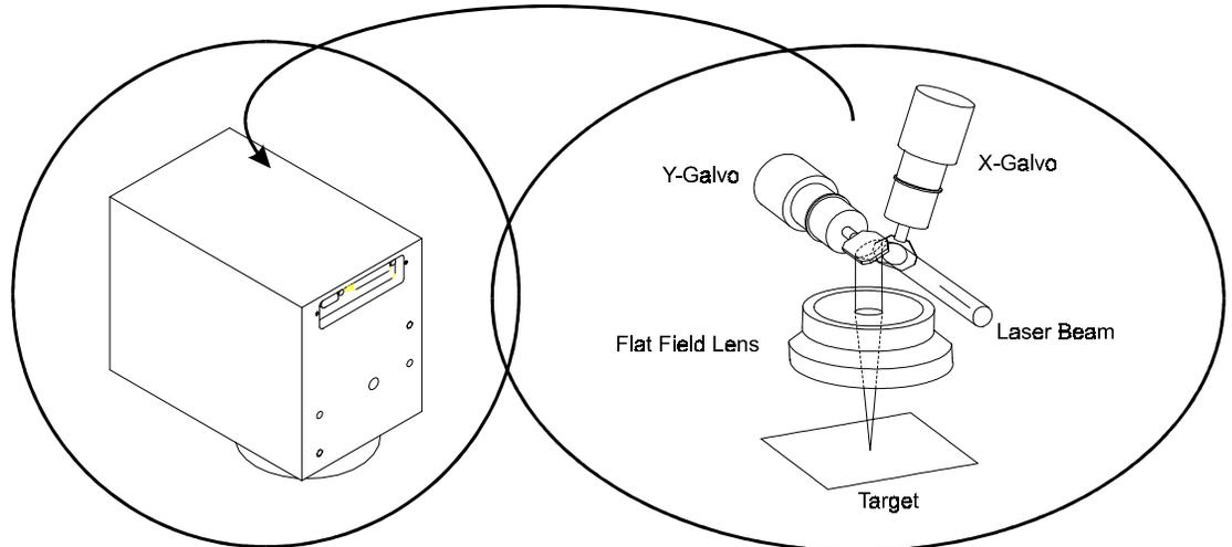
GSI Lumonics' 2-mirror, 2-axis galvanometer Scan Heads provide the capability of deflecting optical beams in an XY manner for all possible laser applications. The synchronized actions of two galvanometer servo-controlled turning mirrors direct the laser beam to specific locations on a target material surface in both the X and Y directions.
