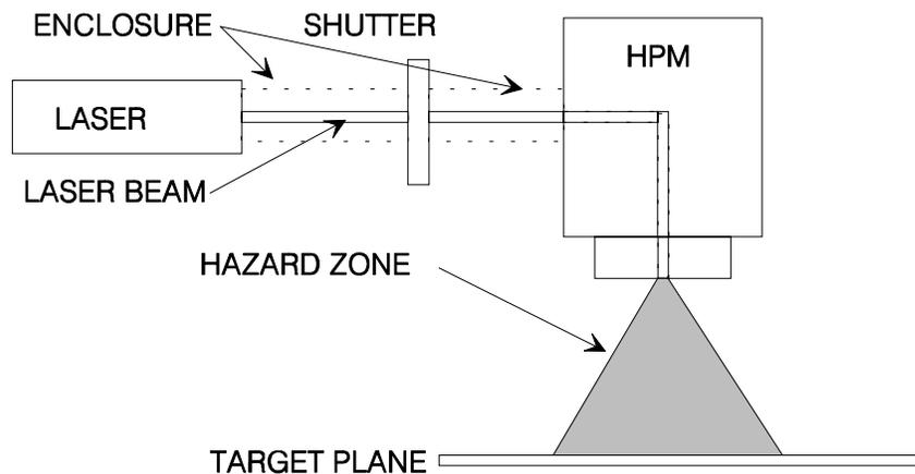
The figure shows the laser's internal and external optical path towards the target plane, specifically where the hazard zones are located as the optical beam passes through as **HPM Scan Head**.
