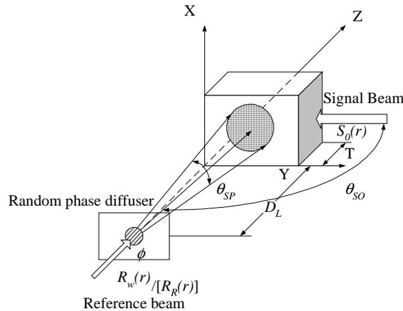
Fig. 1. Geometry of the hologram recording by signal plane wave  $S_0(\mathbf{r})$  and dynamical speckle reference wave  $R_w(\mathbf{r})$ . Here  $T$  is the thickness of volume hologram.  $D_L$  is the distance from the hologram front surface to random-phase diffuser.  $\Delta$  is the shift of the diffuser.
