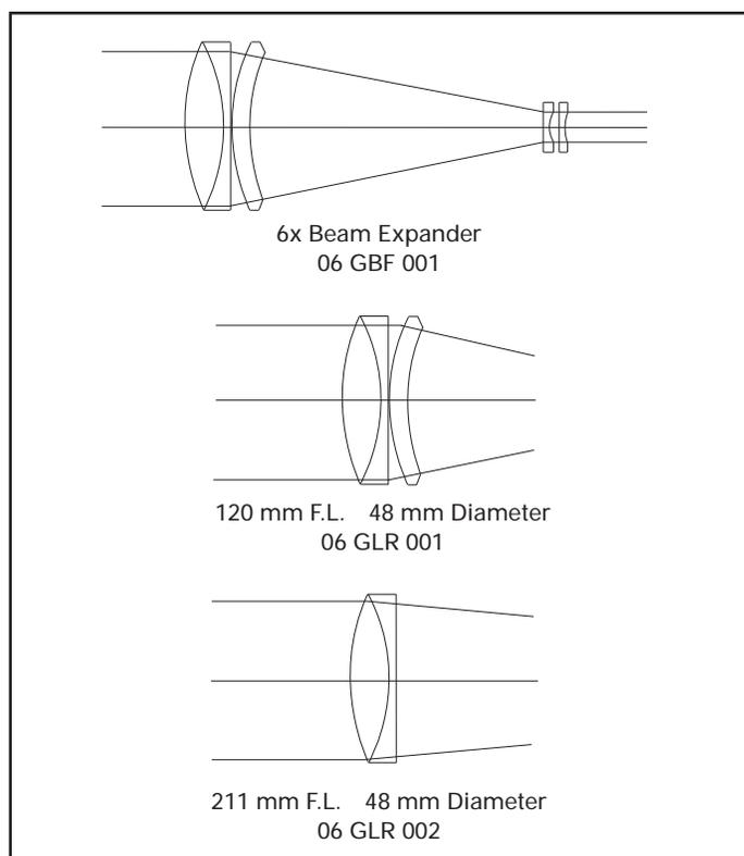
**FIGURE 2. 6 × telescope and receiver lenses.**
