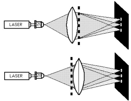
**Viewing diffraction patterns with the eye:**
