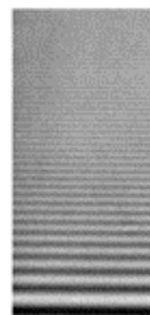
Diffraction pattern formed by a horizontal knife edge.
