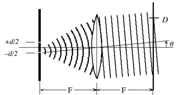
That is, the lower slit emits a cylindrical wave that the lens transforms into a tilted plane wave with an angle  $\theta = \tan^{-1}(d/2F) \approx \sin^{-1}(d/2F)$ . This creates a phase increase of  $\phi = 2\pi (x/\lambda) \sin \theta$  in any plane behind the lens, including the back focal plane at  $F$ . The distance  $D$  then follows from  $\pi = 2\pi (D/\lambda) \sin \theta$ , giving our result,  $D \approx \lambda F/d$ .
