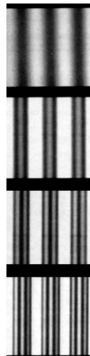
Diffraction patterns produced by 2, 3, 4, and 5 slits.
