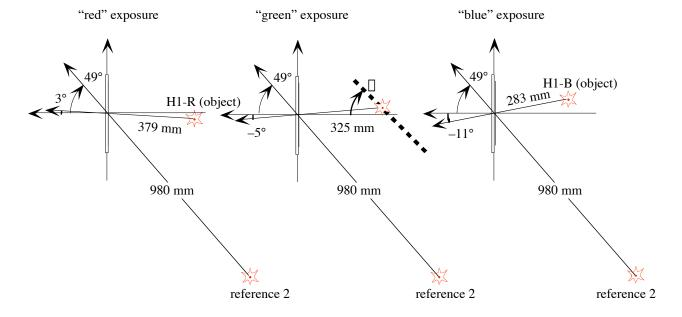
Note that the locations of the slits are on an approximately-straight line tilted at an angle that is the same as the "achromatic angle" derived previously, roughly given by:
