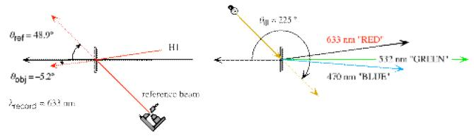
In this case, only the 532 mm green light will be maximally diffracted. The tip angle of the fringes is not quite right for red and blue rays, and even for five micron thick emulsions some falloff due to "Bragg angle mismatching" will be apparent—but not so much so as to detract from the beauty of the hologram.
